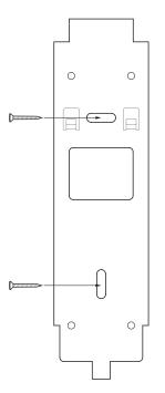
• If installing BioLite N2 on a concrete wall, drill holes, insert PVC anchors, and fix them with fixing screws.
